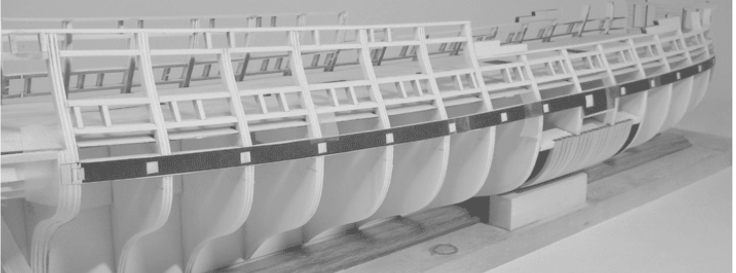
Using the sweep port template to transfer the port openings onto the frames.
