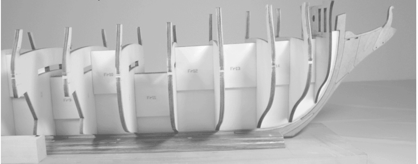
Bulkheads and fillers in place
