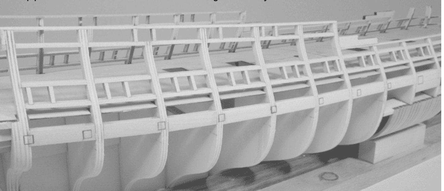
Sweep ports have been transferred to the frames using the stencil you created.
